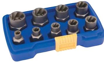
Hanson Bolt Extractors work when everything else fails. They are ideal for rusted or rounded off nuts and bolts. Left hand spiral flutes will tightly grip the damaged fasteners (metric or standard) for quick and easy removal. They have both a 3/8" square drive and hexagonal flats so these extractors can be used with socket wrenches, flat wrenches or impact wrenches. Made from high carbon steel, tougher than tool steel. All sets come in a tough blow molded case for convenient storage.
