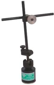
Powerful, permanent magnetic base, 1 1/16" diameter x 1 3/8" high. Fine adjustment for indicator applications. Ball swivel, locks at 90 degree at any position in 360 degree. Center post is 1/4" diameter by 5" high. Cross bar is 1/4" diameter by 5" high.
