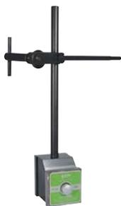
Powerful, permanent magnetic base, 1 7/8" x 1 7/8" x 1 3/8". Furnished with dial indicator Model DI-222 with graduations .001", range .030". Center post is 3/8" diameter by 7 1/2" high. Cross bar is 1/4" diameter by 7" high. Easy on/off push button. Four ground surfaces to grip including V-slot for round surfaces.
