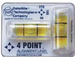
Level has two 360 degree vials with their axis 90 degree to one another. Used for defining warp, machinery base set ups, plumbing, fence posts, RV's, shaft alignment, cameras, and appliances. Fast, simple, repeatable. Magnetic for non-permanent use.
