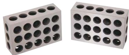
Set of two, features cross drilling design, five holes tapped 3/16 for holding down. 18 holes drilled through. Total of 23 holes on all six sides. Parallel to .0001" overall. Square to .0001" length. Case hardened to HRC 55 to 62.
