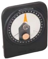
Used for critical projects to accurately set or measure angles. Oil damped, ball bearing movement does not stick, vibrate or bounce. A strong magnetic base allows hands-off use on ferrous metals. Dial is 2.6" diameter with vernier divisions of 1/10". Outside dimensions are 3.6" x 3.1". Includes case.
