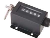
Counters advance one count for each complete revolution of shaft. Maximum speed 1,000 counts per minute. White numerals on black background. No lubrication required. Deluxe model has metal internal parts. Economy model contains plastic internal parts.
