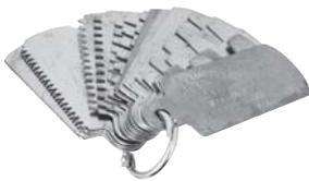
This handy, steel gear gauge set consists of 16 leaves, 24 gauges, to measure both 14 1/2 degree and 20 degree pressure angle tooth form, in diametral pitch sizes 64, 48, 32, 24, 20, 16, 12, 10, 8, 6, 5 and 4. Pitch sizes 8, 6, 5 and 4 both 14 1/2 degree and 20 degree are cut on individual leaves. Pitch sizes 64 through 10 inclusive, have both 14 1/2 degree and 20 degree pressure angles on a single leaf.
