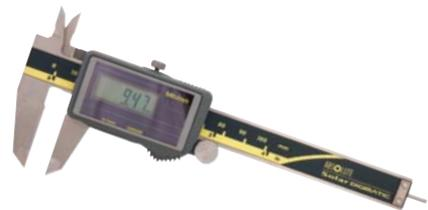
Digimatic calipers with solar cells which gather light energy and convert it to power. Eliminates the need for battery replacement. When ambient illumination is over 125 lux., the surplus power is stored. It can be run for approximately three hours after fully charging.
