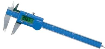
MyCal Lite is an innovative new digimatic caliper which is economically priced to allow everyone to benefit from the advantages of modern digital gauges. Large .3" LCD digits ensure error free reading in either inch or millimeter mode. Zero point can be set anywhere to allow comparison measurements. Accuracy ±.005". Response speed 63" per second. One SR44 battery supplied. Battery life is approximately two years under normal use. Over speed and low voltage alarms. Includes a depth bar.
