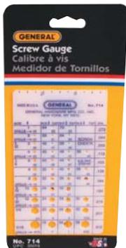
Quick way to identify machine screws, bolts, wood screws, self-tapping screws, standard size rivets and common cotter pin sizes up to 3/16" (8mm). 3" scale to check screw lengths. Checker gives required drill size for corresponding tap size and proper drill size for like hole. Threaded holes indicate threads per inch while unthreaded indicate size by number and fractions of an inch. Durable engineering plastic.
