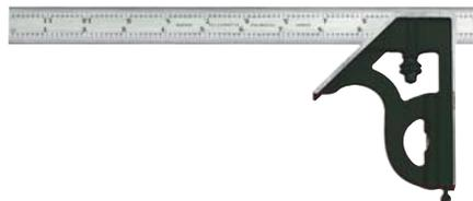
Combination squares with reversible lock bolts, scriber, spirit level, and hardened steel, machine-divided blade with regular finish. Cast iron heads with black wrinkle finish.
