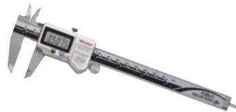
These digital calipers have a sealed housing and are IP-67 rated, meaning it is nearly immune to the coolants, dirt, grit, and chips found in many manufacturing environments. Features a measuring range from 0 to 6"(0-150mm) with a resolution of .0005"(0.01mm). Accuracy is ±.001" inch/metric with no SPC output.
