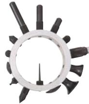
Fourteen points with #4-48 screw thread to fit AGD dial indicators. Includes: one regular 1/4" long point, nine special form points, one No. 28 shock absorbing anvil and three extra long points (1/2", 3/4" and 1"). All are made of high grade hardened steel. Mounted on an aluminum ring for easy selection and safe keeping.
