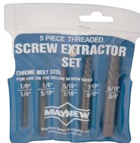
Spiral thread design allows quick and easy removal of broken bolts, screws and pipe studs. Simply drill and insert extractor. No hammer is needed. The set includes 5 extractors to remove bolts from 1/8" to 3/4". Tip diameters .095", .140", .185", .243" and .335"
