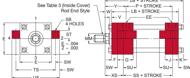
**TABLE 1LH** The dimensions given on this table are affected by the piston rod diameter and the stroke.
