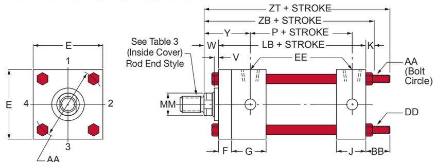
**TABLE 1LH** The dimensions given on this table are affected by the piston rod diameter and the stroke.
