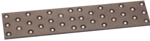
Used for handling large work in drill presses or band saw machines. Placed between work and the machine so that the work can easily be moved. All are black oxide finish with 3/8" diameter hardened steel balls. Balls are exposed on both sides of parallel. Parallel is 1/4". Load capacity is 3,000 lbs. per ball.
