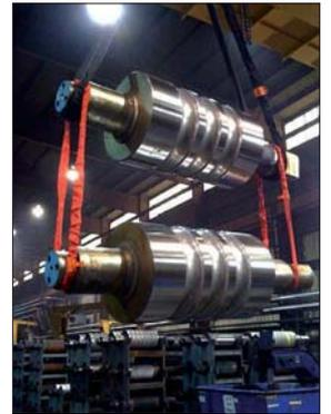
Round slings have a double wall cover for greater life and added protection. Wear points can be shifted to extend life of the sling. Chokes tighter and releases easier than other slings. Color coded for rated capacity. Has red core warning yarn inspection system.
