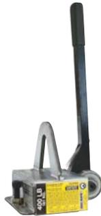
Ideal for handling steel plates, forgings, die castings. **Should only be used for thick, non-flexing ferrous materials.** Eliminates need for slings, clamping devices or chains. Lifting magnets offer the safety of a permanent lift. Strong eye bolt for lifting, quick cam action release handle for on/off.
