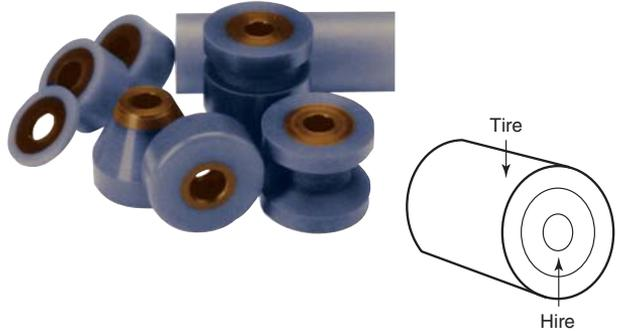
Made from K-prene™ urethane. Low cost alternative for wheels, casters, rollers, sheaves, etc. Blue outer tire (90A durometer) is bonded to a brown hub (75D durometer), resulting in a hard anti-friction bearing with a softer outer tire. Can serve as a bearing in some applications. Comes in 12" and 24" lengths. Cut to fit your application.
