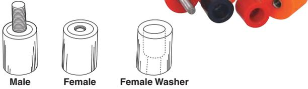
These bumpers feature steel cores with male or female threads. Washers have counterbored holes to accept socket head cap screws and a flat washer molded inside.
