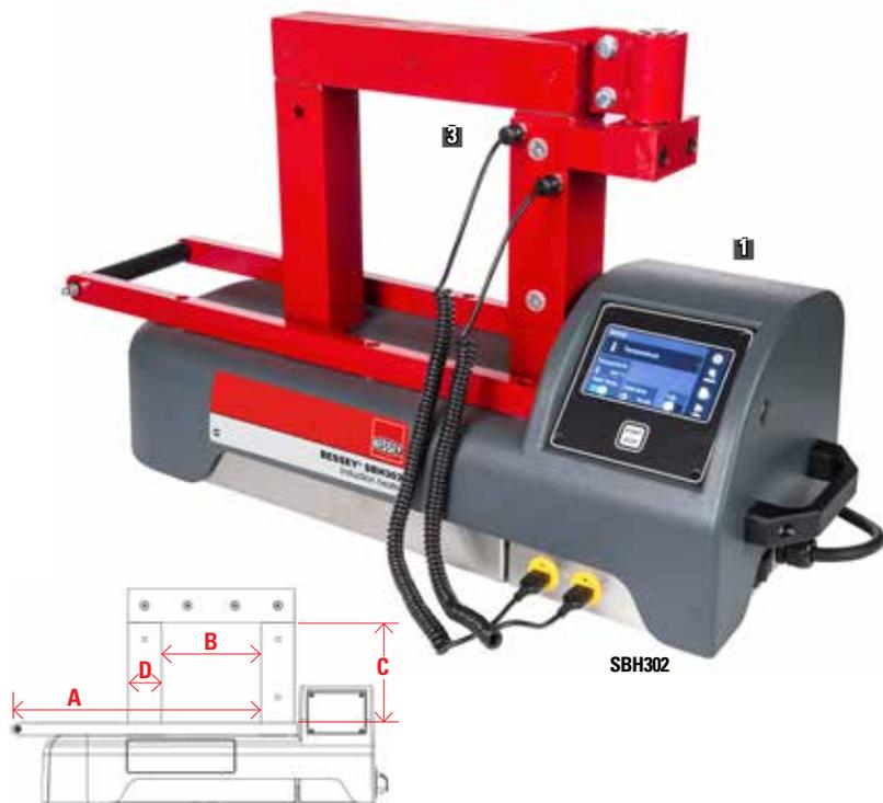
Proper bearing installation is essential to maximum bearing life. By heating prior to installation, the bearing expands and slides easily onto the shaft. Magnetic induction is a safe and efficient method of generating heat to expand bearings for installation. No open flame or hot oil to worry about. Magnetic induction heats bearings evenly and quicker than hot plates.
