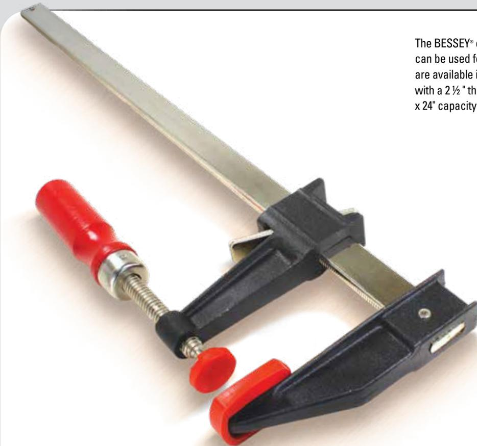
The BESSEY® clutch style clamps are a popular regular duty clamp that can be used for a wide range of projects. These economical clamps are available in a wide range of sizes starting with the GSCC2.506 with a 2 ½" throat x 6" capacity up to the GSCC5.024 with a 5" throat x 24" capacity and, a range of clamping force from 600 to 1200 lbs.
