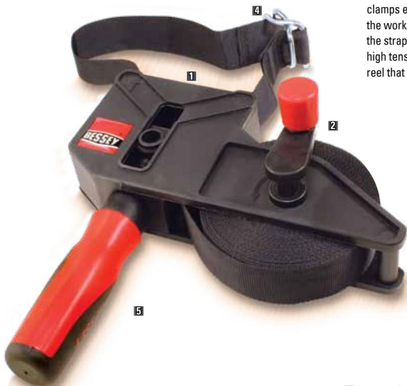
Clamping large or odd shapes with straps is not new; however, most strap clamps exert force (pull) in only one direction which can easily distort/skew the work piece. BESSEY's VAS-23 is different, it pulls equally on both ends of the strap, eliminating the chance of skewing your work piece to one side. The high tensile woven polyester strap is extremely strong with a built-in take up reel that neatly stores the excess strap; eliminating a potential tripping hazard.
