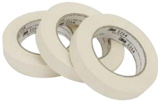
Economical, quality, general purpose paper tape with rubber adhesive. Exceptional shear to corrugated boxes and exceptionally consistent adhesion. Use for bundling, sealing, holding and non-critical indoor jobs. 5.3mil, pressure sensitive tape resists slivering. Use up to 150 degree Fahrenheit.
