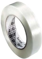
Clear polypropylene film backing reinforced with glass yarn filaments. High tensile strength, nick resistance, abrasion resistance and good handling for utility bundling, reinforcing, and pallet unitizing applications.
