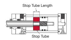
The stop tube is located between the piston and the rod end cap. It limits the extended stroke of the cylinder, providing additional strength for less cost and reduced weight than the use of an oversize rod.
