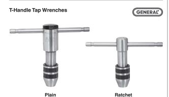
Provides good leverage in tight spaces. Holds taps, reamers, screw extractors and hand held tools. Self-centering hardened tool steel and knurled chuck sleeve provide positive grip. Ratchet wrenches can be set for right or left hand operation or locked for non-ratchet use.
