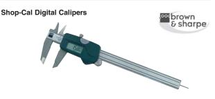
These calipers provide easy to read accurate measurements of day to day operations. Stainless steel for durable, reliable and accurate measurements. Features a resolution of .00005" (0.01mm) with specifications consistent with DIN 862. Its power supply is a 3V lithium battery and auto shut-off for superior longevity. Instant inch/metric conversion.
