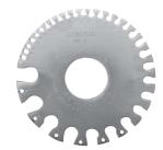
For gauging uncoated sheet metal, plate iron and steel.
