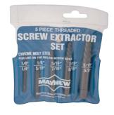
Spiral thread design allows quick and easy removal of broken bolts, screws and pipe stubs. Simply drill and insert extractor. No hammer is needed. The set includes 5 extractors to remove bolts from 1/8" to 3/4". Tip diameters .095", .140", .185", .243" and .335"
